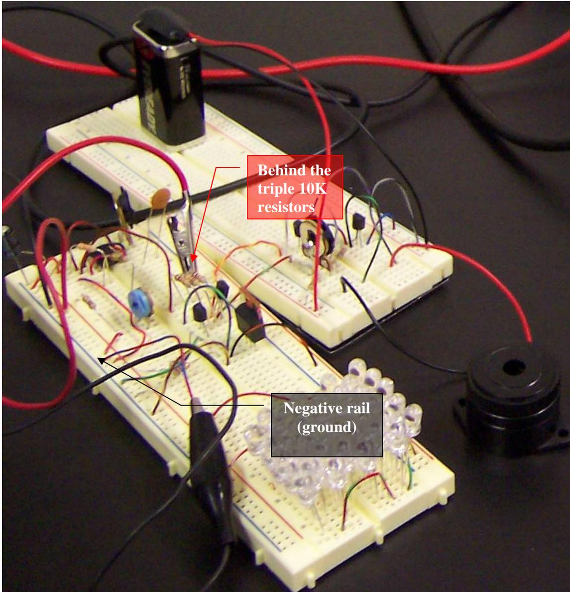
Connect the red terminal to where the red box is pointing to. Connect the black terminal to ground.
