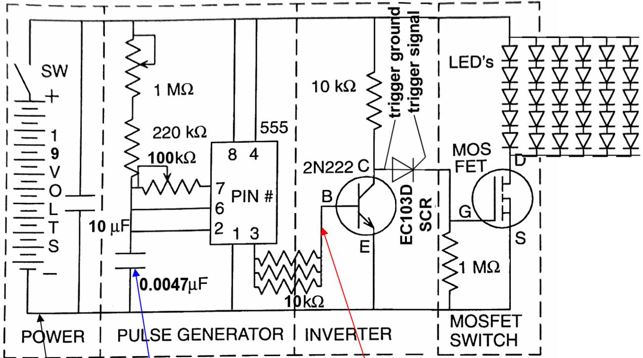
Highlighted are best places to place oscilloscope probes.
